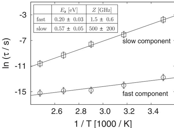
FIG. 3. Arrhenius plot of the characteristic lifetimes for the fast and slow component of the decay of the light-induced absorption at  $\lambda = 785$  nm ( $I_p = 13.5$  GW/m<sup>2</sup>).
