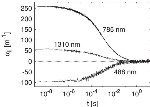
FIG. 1. Temporal development of the light-induced absorption for the three probe wavelengths at  $T = 315 \text{ K}$  and maximum pump intensity of  $I_p = 670 \text{ GW/m}^2$ .
