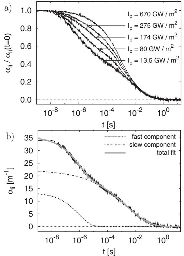
FIG. 2. (a) Temporal development of the light-induced absorption for a probe wavelength  $\lambda = 785 \text{ nm}$  for different pump intensities at  $T = 315 \text{ K}$ . The spectra are normalized to their maxima for reasons of comparability. (b)  $\alpha_{li}(t)$  for  $I_p = 13.5 \text{ GW/m}^2$ . The lines are fits of stretched exponential functions [see Eq. (1)] to the experimental data.
