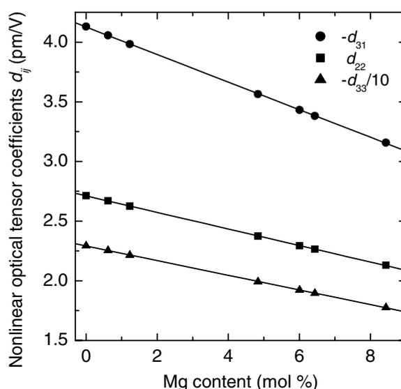
**Figure 4.** Dependences of the second-order nonlinear optical tensor coefficients  $d_{ij}$  of Mg-doped LiNbO<sub>3</sub> crystals at 1.079  $\mu\text{m}$  on the Mg concentration in the crystal.
