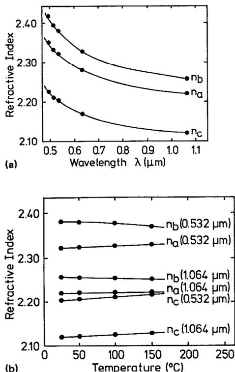
FIG. 1. (a) Dispersion of KNbO<sub>3</sub> at room temperature. (b) Temperature dependence of the refractive indices of KNbO<sub>3</sub> at 532 and 1064 nm.<sup>5</sup>
