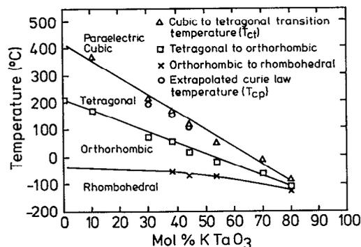
FIG. 2. Dependence of the phase transition temperatures of KNb<sub>1-x</sub>Ta<sub>x</sub>O<sub>3</sub> from the Ta concentration.<sup>4</sup>
