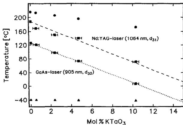
FIG. 5. Temperatures for noncritically phase-matched SHG vs Ta-concentration (squares) for Nd:YAG- and GaAs-laser. Circles and triangles indicate the orthorhombic→tetragonal phase transition and the orthorhombic→rhombohedral phase transition, respectively (calculated from Ref. 4).
