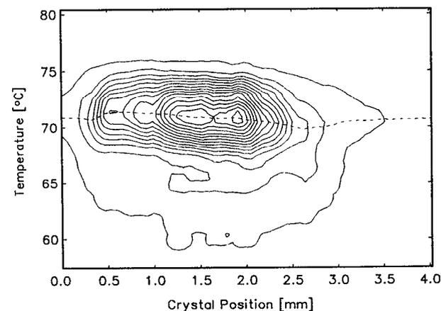
FIG. 4. Contours of constant intensity of the spatially resolved SHG measurement of KNb<sub>1-x</sub>Ta<sub>x</sub>O<sub>3</sub> with a Ta concentration of 10.3%. The dashed line shows the phase-matching temperature versus crystal position.
