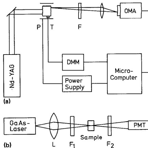
FIG. 3. (a) Experimental setup for spatially resolved SHG with Nd:YAG-laser (OMA: optical multichannel analyzer, P: peltier-cooling/heating, T: thermocouple, F: short-pass filter BG 18). (b) Setup for phase-matched SHG with GaAs-laser (L: focusing lens, F1: interference filter for 905 nm, F2: short-pass filter BG 18).
