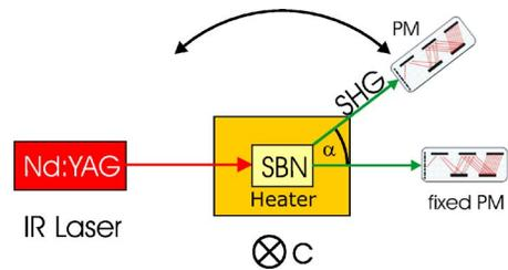
FIG. 3. (Color online) Setup for quantitative measurements: the infrared light hits the temperature-controlled crystal perpendicular to its  $c$  axis. The generated harmonic light is detected by two photomultipliers. One is rotated by a motorized stage around the crystal, the second one is mounted at a fixed angle of 0° with respect to the fundamental beam.
