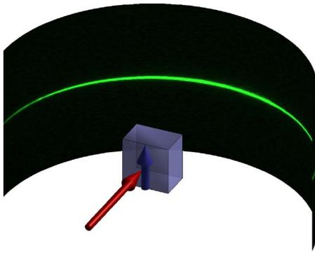
FIG. 2. (Color online) Principle of the measurements: a Nd:YAG laser beam (long arrow) is directed onto an SBN crystal in a direction perpendicular to the crystallographic  $c$  axis (short arrow). A photograph of the emitted SHG light pattern for an unpoled sample is shown on the screen.
