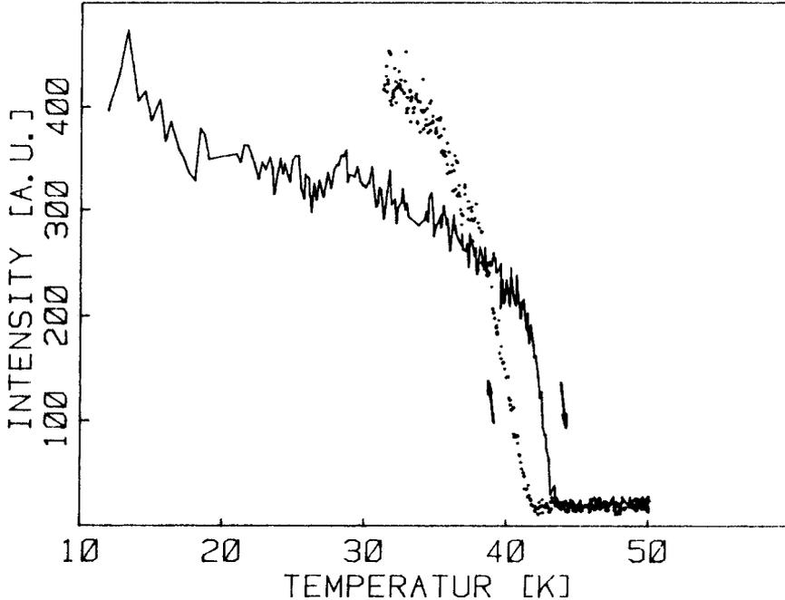
FIGURE 1 SHG-signal in  $\text{KTaO}_3:\text{Li}$  as a function of the sample temperature.
