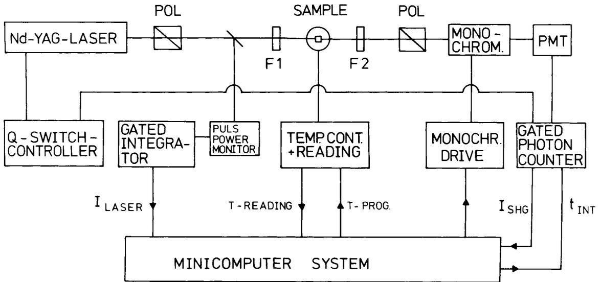
Figure 1: Experimental setup for measuring the temperature dependence of the SHG intensity in  $\text{SrTiO}_3$ . F1 and F2 are IR-edge (Schott RG 830) and IR-blocking filters (Schott BG 18), respectively.
