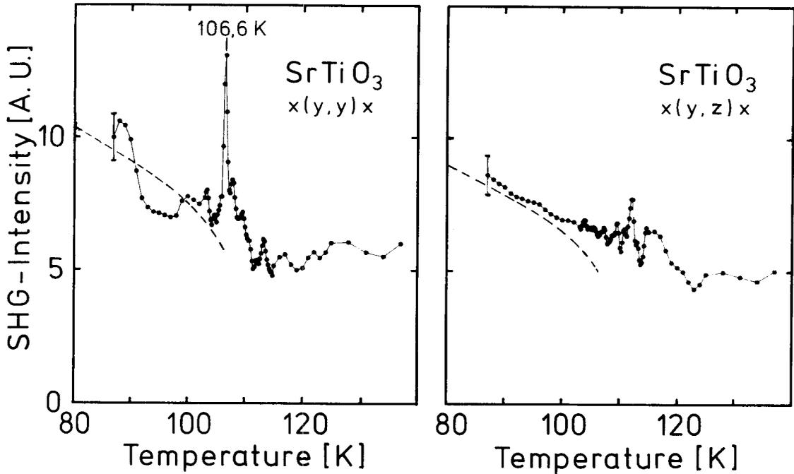
Figure 2: Temperature dependence of the SHG intensity in SrTiO<sub>3</sub>, second harmonic polarization parallel (left) and perpendicular (right) to the fundamental beam polarization. The measured values are given by the dots, typical measurement errors are indicated by the bars.
