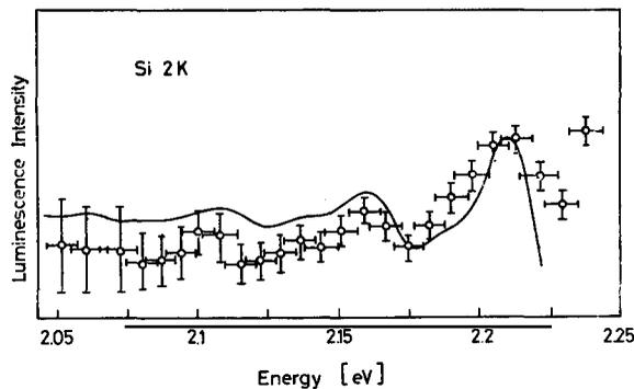
FIG. 2. Luminescence spectrum below  $2E_g$  with better resolution. The full line gives the theoretically expected shape (ratio of optical to acoustical relaxation rate: 2.7).
