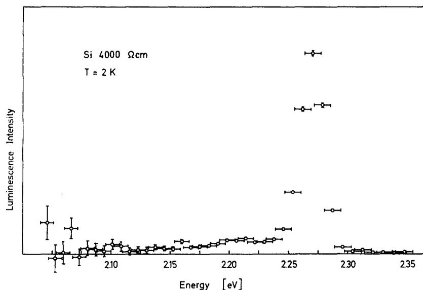
FIG. 1. The near- $2E_g$  luminescence spectrum of GaAs-laser excited silicon. The relatively intense line at 2.27 eV is caused by two-electron transitions in the EHD.
